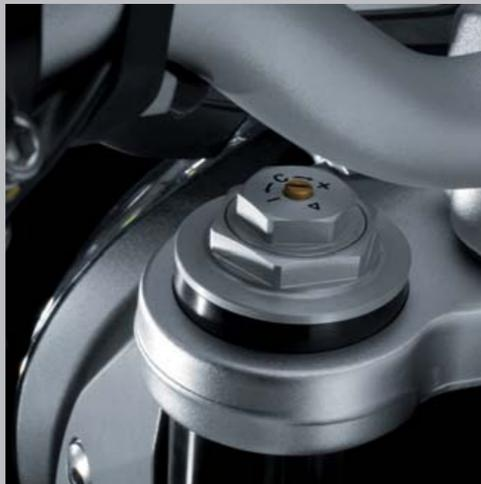
At MV Agusta we realise how important it is to personalise your bike to get the maximum performance from your machine resulting in perfect road handling. The Brutale 800 front suspension is fitted with adjustability for rebound, preload and compression, tailored handling is just a click away for easy and immediate results to ensure the ultimate ride on road or track. MV Agusta, always offering you more to enjoy !
